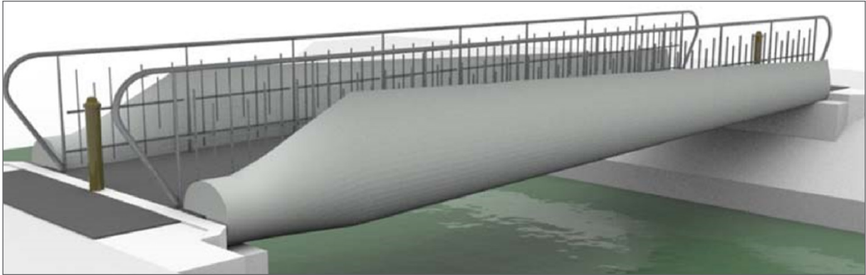
A conceptual design of pedestrian bridge using A29 wind blades as main girders, Re-Wind research project [24]
