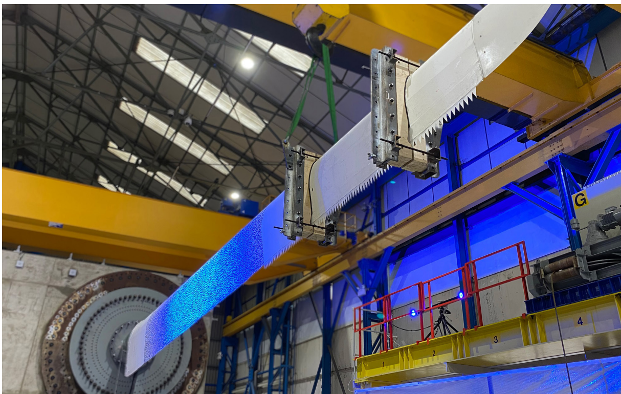
FIGURE 10 Automated testing for wind turbine blades
